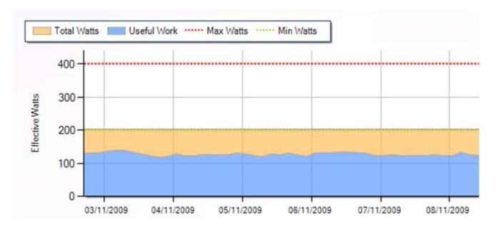
As you can see from the legend, the orange section represents the total Watts of power the server is consuming. This server is currently consuming approximately 200 Watts of power but at peak load could consume up to 400 Watts as denoted by the green and red dotted lines. The blue section represents the calculated useful work the server is performing. This server is considered well utilized as there is typically more than 50% useful work.
