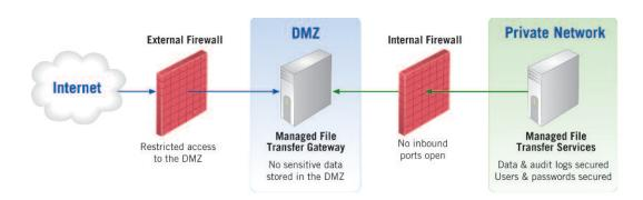
A DMZ gateway functions as both a reverse and forward proxy, keeping sensitive data out of the public-facing DMZ, masking private network addresses, and leaving inbound ports closed to the internal network.
